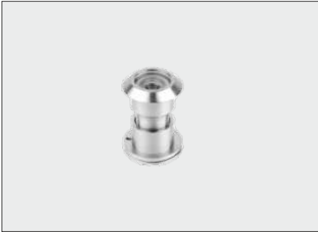
HDV1: Door Viewer ► Lens diameter: 37 mm, Lens cone diameter: 22 mm ► Suitable for door thickness: 35 – 55 mm ► 180°view, nylon with cover plate from indoor side ► Finishes: Chrome/ Antique Brass/ Black
