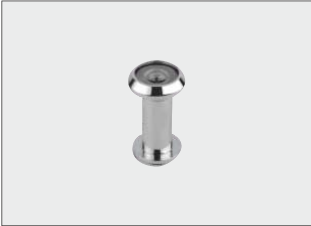
HDV 2: Door viewer ► Lens diameter: 25.4 mm, Lens cone diameter: 14 mm ► Suitable for door thickness: 35 – 60 mm ► 140°view, nylon with cover plate from indoor side ► Finishes: Chrome/ Antique Brass/ Black
