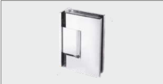
HGC 05: 90° Wall to Glass Fix Clip Connector ► Passed 96 hours Salt spray test ► Base material: Brass ► Finish: Bright Chrome
